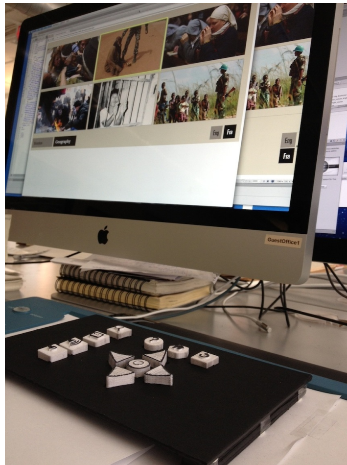
Figure 3. User testing setup showing testing prototype keypad with interactive interface.
