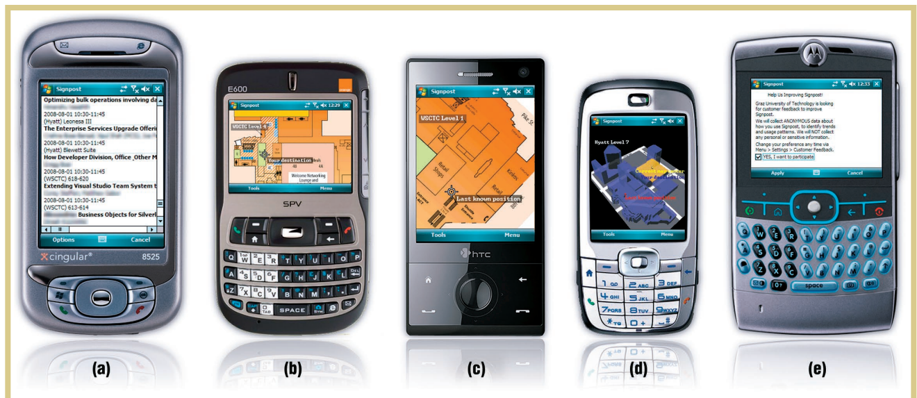
Figure 3. Examples of phones running Signpost and screenshots of the application: (a) HTC Cingular 8525, (b) Orange SPV E600, (c) HTC Touch Diamond, (d) HTC S710, and (e) Motorola Q. Signpost supports various form factors and resolutions of the screen, and different input capabilities (both keypad- and touch-based).
