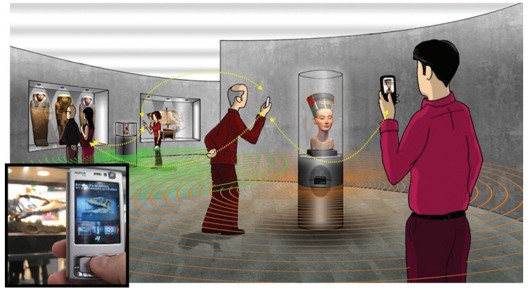
Figure 1. The basic concept of the PhoneGuide system in a museum. Our system uses adaptive classification in dynamic large-scale museum environments. Ad hoc sensor networks and phone-to-phone communication support PhoneGuide.
