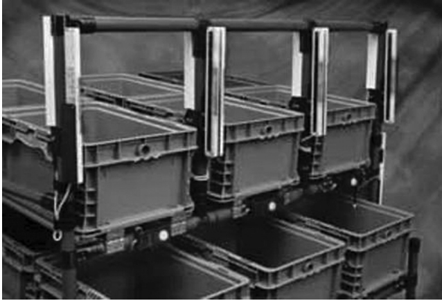
Figure 10.4 A just-in-time inventory cart is instrumented with light curtain sensors. When a worker's hand enters the bin to get a part, it breaks the light beam. There is a light beneath each bin. If the assembly process uses barcodes or RF tags to identify an assembly, a processor controller can activate the light on the bins with the correct parts for that assembly.
