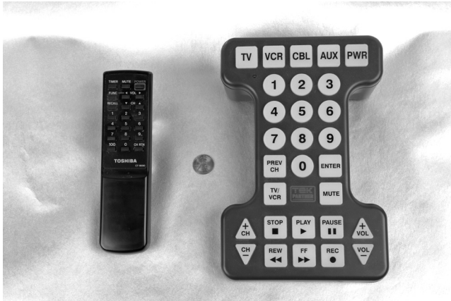
Figure 7.1 Two remote control units. The one on the right was designed to be more accessible. The device is larger with larger control buttons that are back-lit when a button is depressed.
