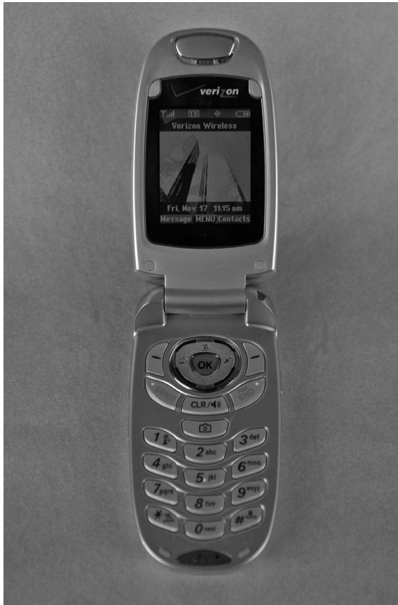
Figure 8.13 Typical small flip-open mobile phone. The keys on the keyboard are small, and the display is small, usually packed with a large amount of visual information.
