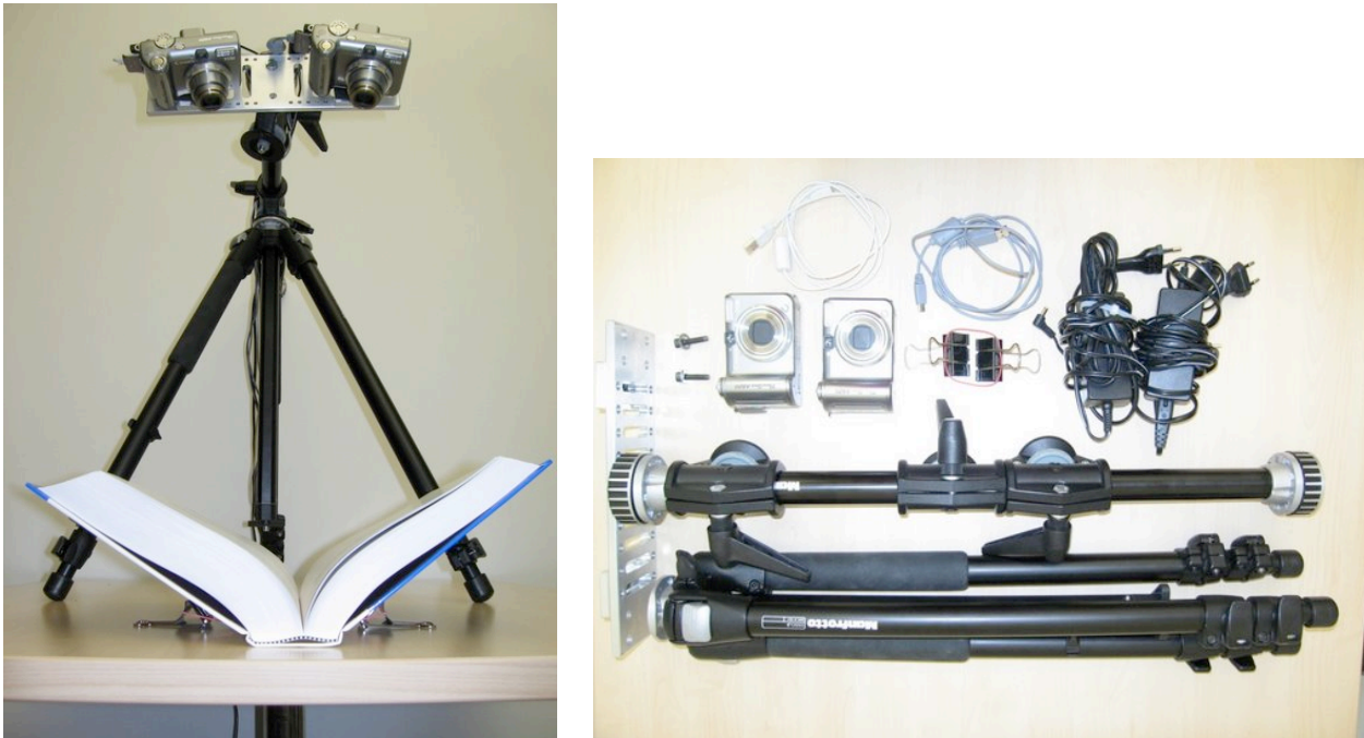
Figure 1: A prototype scanning rig, consisting of standard tripod hardware and consumer digital cameras. The rig is portable and can be operated anywhere using a laptop computer.
